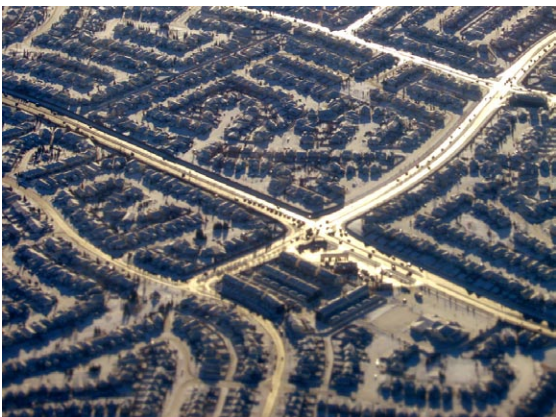
Figure X. From the air one can easily see the difference between heavy traffic arterials and light traffic cul-de-sac
