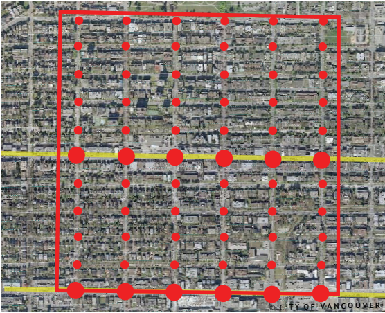
Figure X. This typical sq km in Vancouver, British Columbia has 66 intersections
