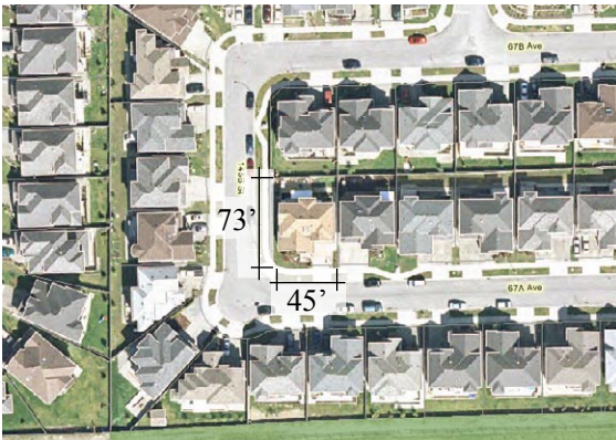
Figure X. The aerial photograph taken in Surrey, BC shows shallow lots with large frontages dominated by driveways
