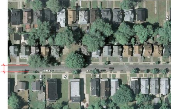
Figure X. Cleveland: 24' curb to curb width
